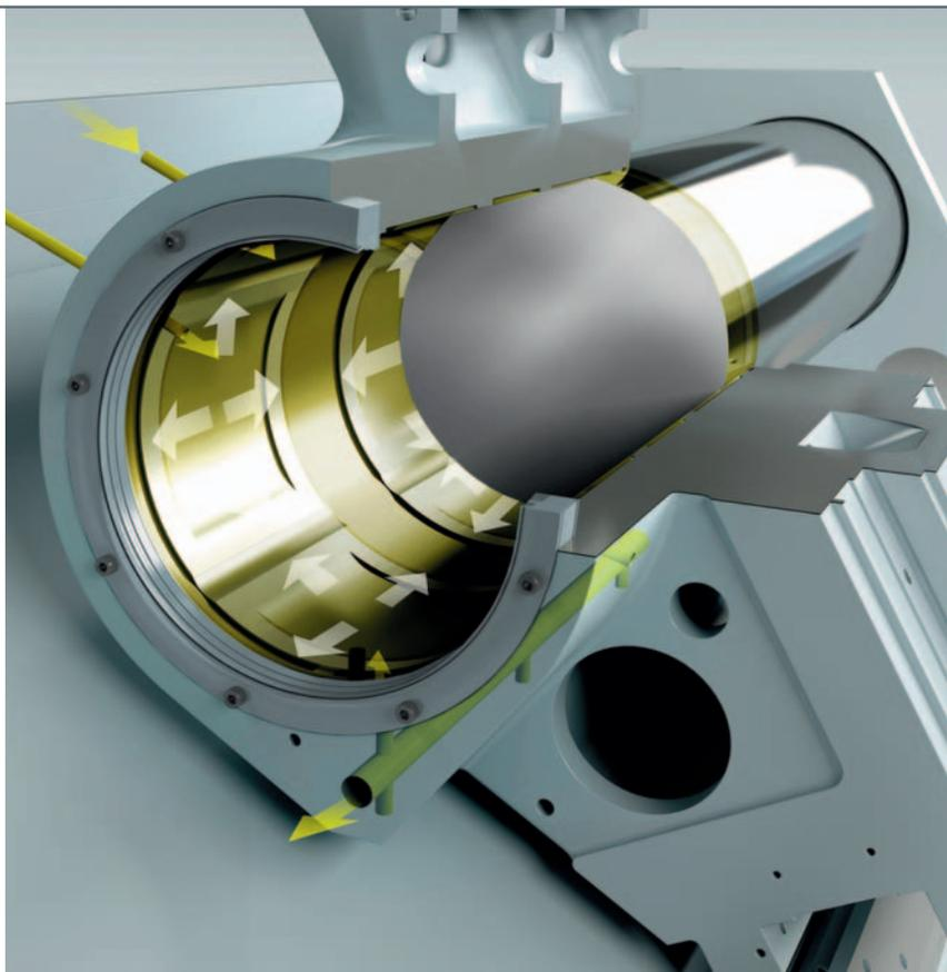
2 Hydrostatic column guide with highest damping
